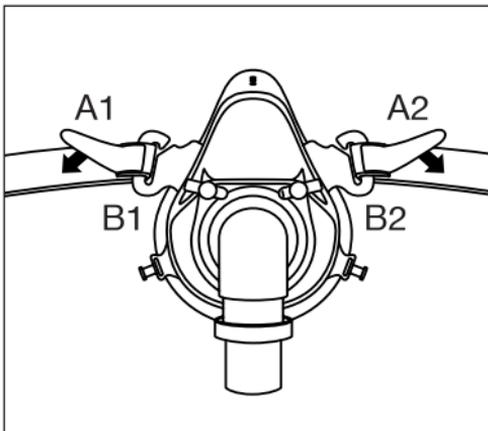
Pull the upper straps of the headgear A1 and A2 through the slots in the forehead support B1 and B2. Make sure that the the Velcro is faces outward. Fix both Velcro tapes.
