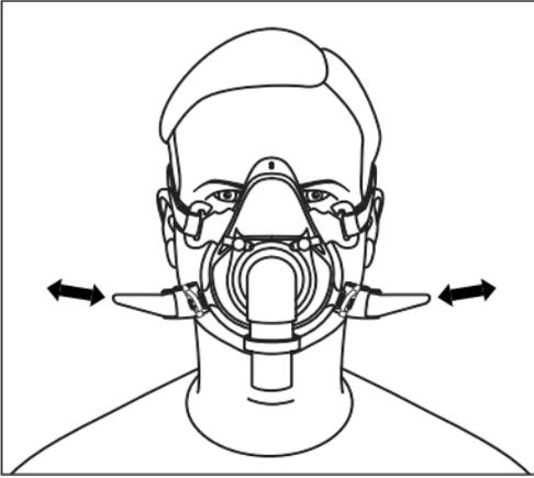
Adjust both lower headgear straps A3 and A4 to a comfortable tension.
