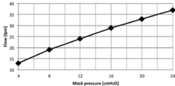
*N.B. Due to manufacturing differences, the exhalation flow rate may differ from the values shown in the table ( $\pm 10\%$ ).*
