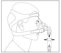
Press the two holding clamps of the quick release connector together and disconnect the tube from the mask.
