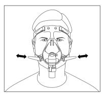
Adjust both lower headgear straps A3 and A4 to a comfortable tension.
