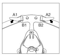
Pull the upper straps of the headgear A1 and A2 through the slots in the forehead support B1 and B2. Make sure that the the Velcro is faces outward. Fix both Velcro tapes.
