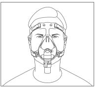
Hook the buckles A3 onto B3 and A4 onto B4 on mask frame.
