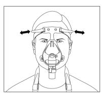
Adjust the upper headgear straps A1 and A2 to a comfortable tension.
