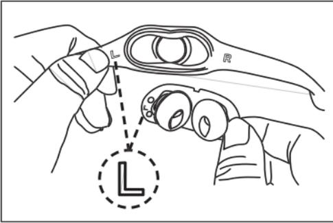
Attach the pillow set into the main frame. Make sure the platform concave is fitted to the main frame protrusion.
