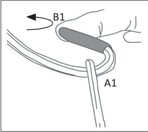
Insert the Velcro strap B1 into A1 and fasten it.
