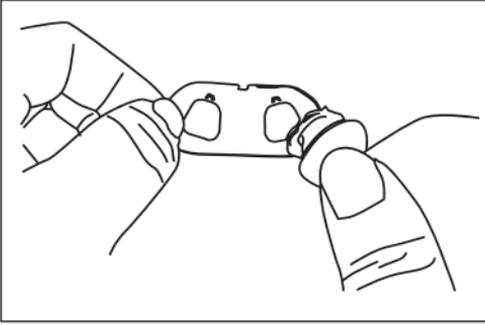
Attach the pillows on the platform. Make sure the tenons are fitted.
